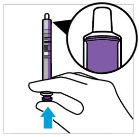
Push plunger all the way in to remove air.
